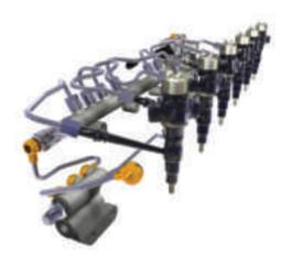
**XPI Fuel System** – The proven technology of the XPI common-rail fuel system delivers a precise quantity of fuel at ultra-high pressures. This, together with more robust electronic engine controls, enables multiple injection events per cycle. Flexibility in injection timing increases fuel economy and performance while decreasing exhaust emissions.
